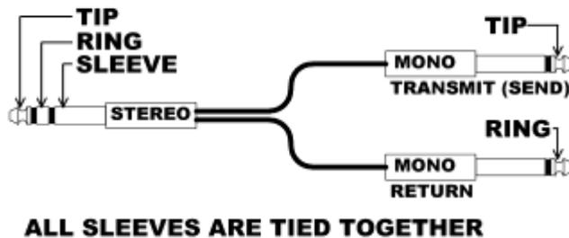
The TRS insert cable is used to patch in external effects into the WET2 signal path. The TRS end transmits the wet signal from the Growler via the TIP and the signal is returned via the RING of the plug.
