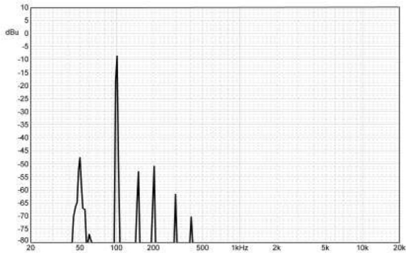
Fundamental signal input -10dBu @ 50Hz. WET and DRY levels set to unity.
